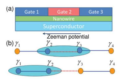
$$H = \left[\zeta_{12}\alpha(t)\gamma_1\gamma_2 + \zeta_{23}(1 - \alpha(t))\gamma_2\gamma_3\right]$$
