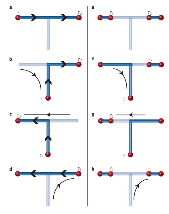
A trijunction between two topological nanowires is potentially a more complex topological object than the simple topological nanowire. The continuous transport of MFs through such a trijunction is potentially dependent on details of the junction that may be difficult to control.
