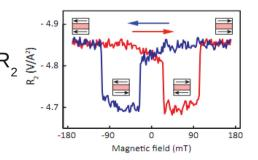
→ Measured effect at 300K is spin Peltier effect
