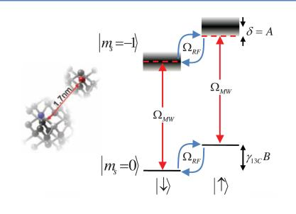
In the presence of a <sup>13</sup>C nuclear spin, one expects an additional collaps in the signal at time  $~t= au=\pi/A_{\parallel}$  , for which one finds  $\langle m_s
