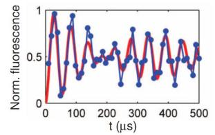
In this sample, around 1 out of 10 NV centers had a  $^{13}$ C nuclear spin close by (1-2 nm). Here:  $\sim 1.7$  nm
