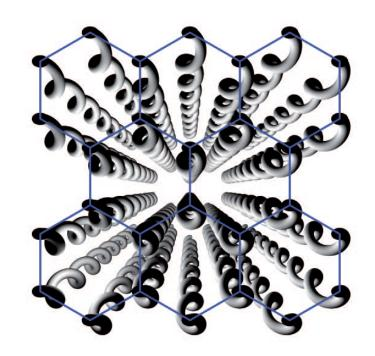
The photonic lattice is an array of evanescently - coupled waveguides arranged in a honeycomb structure with nearest-neighbor spacing of 15  $\mu$ m
