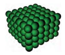
Examples of 1D, 2D and 3D photonic crystals: Bragg grating, porous silicon, opal.
