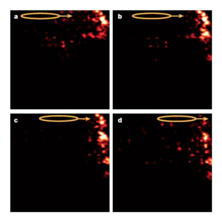
to the right in a-d. The beam propagates along the top edge of the array (which is in the zig-zag configuration), hits the corner, and clearly moves down the vertical edge (which is in the armchair configuration). Note that the wavepacket shows no evidence of backscattering or bulk scattering due to its impact with the corner of the lattice. This scattering of the edge state is prevented by topological protection.
