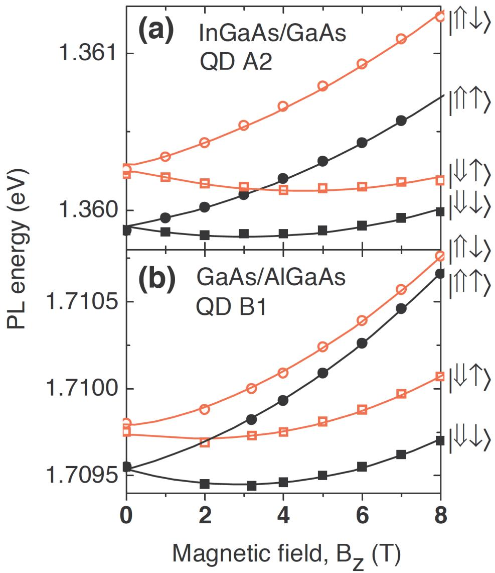
Magnetic field dependence of exciton PL Energies in InGaAs QD (a) and GaAs QD (b).
