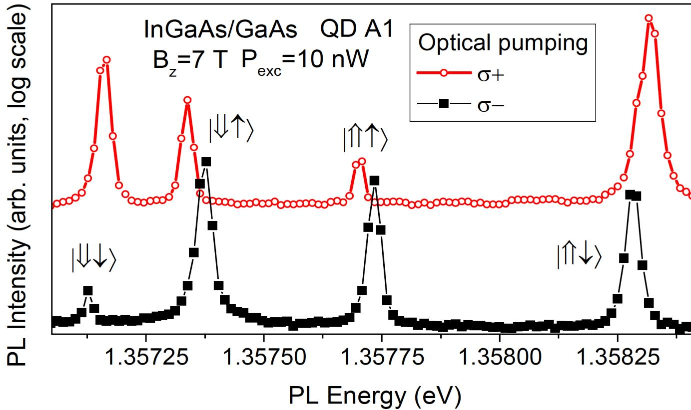
Nuclear spin polarization shifts excitons with electron spin  $\uparrow(\downarrow)$  to lower (higher) energies.
