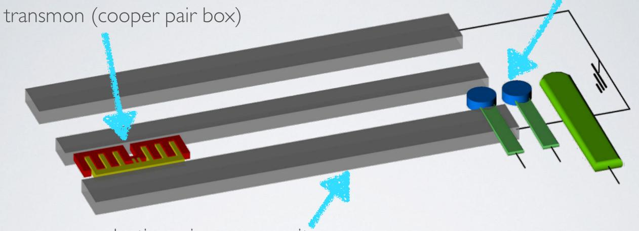
superconducting microwave cavity
