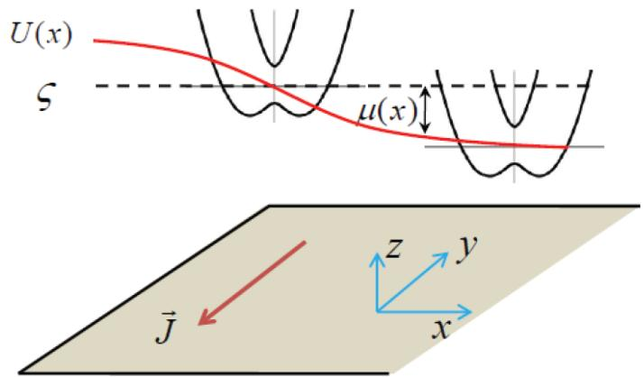
The smooth potential  $U(\mathbf{R})$  determines the position of the bottom of the band
