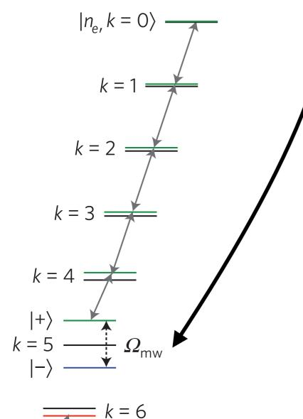
• Selectively addressing one of the spin states with 'Zeno' continuous MW resonant on the transition  $|n_e,k_z\rangle \rightarrow |n_q,k_z\rangle$
