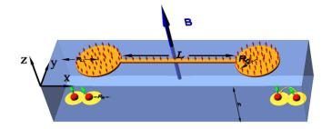
Via capacitive coupling through floating gates (long-distance)
