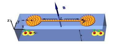
Via capacitive coupling through floating gates (long-distance)
