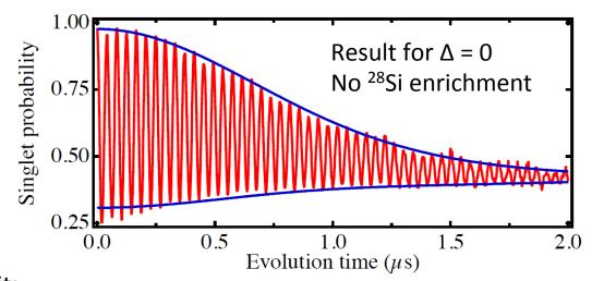
Fit: Double Gaussian decay with 1/e decay time of 1.0  $\mu$ s for hyperfine interactions and 1.5  $\mu$ s due to charge noise
