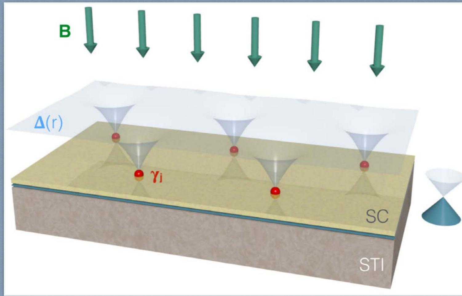
Superconducting order is induced in the surface of a strong topological insulator (STI). Magnetic field **B** induces Abrikosov vortices in the SC order parameter. Each vortex hosts an unpaired Majorana zero mode  $\gamma_j$ .
