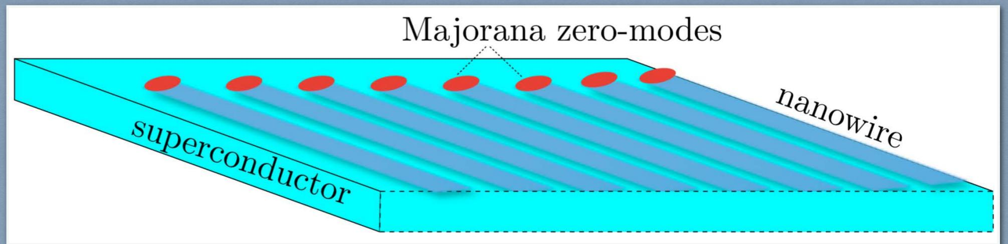
Array of nanowires on a superconducting substrate, with a delocalized Majorana edge mode composed out of coupled zero-modes localized at the end points.
